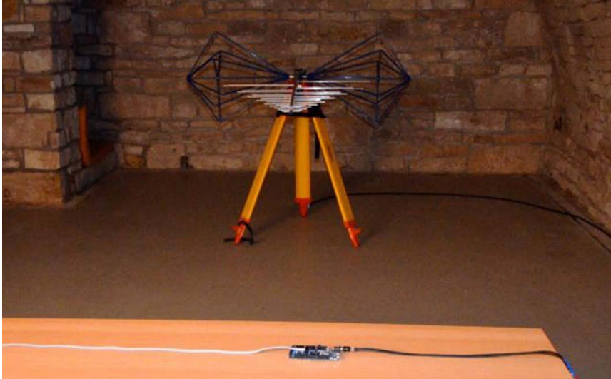
Figure 3: Setup of the far-field measurement - antenna at a distance of 3 m from the circuit board
